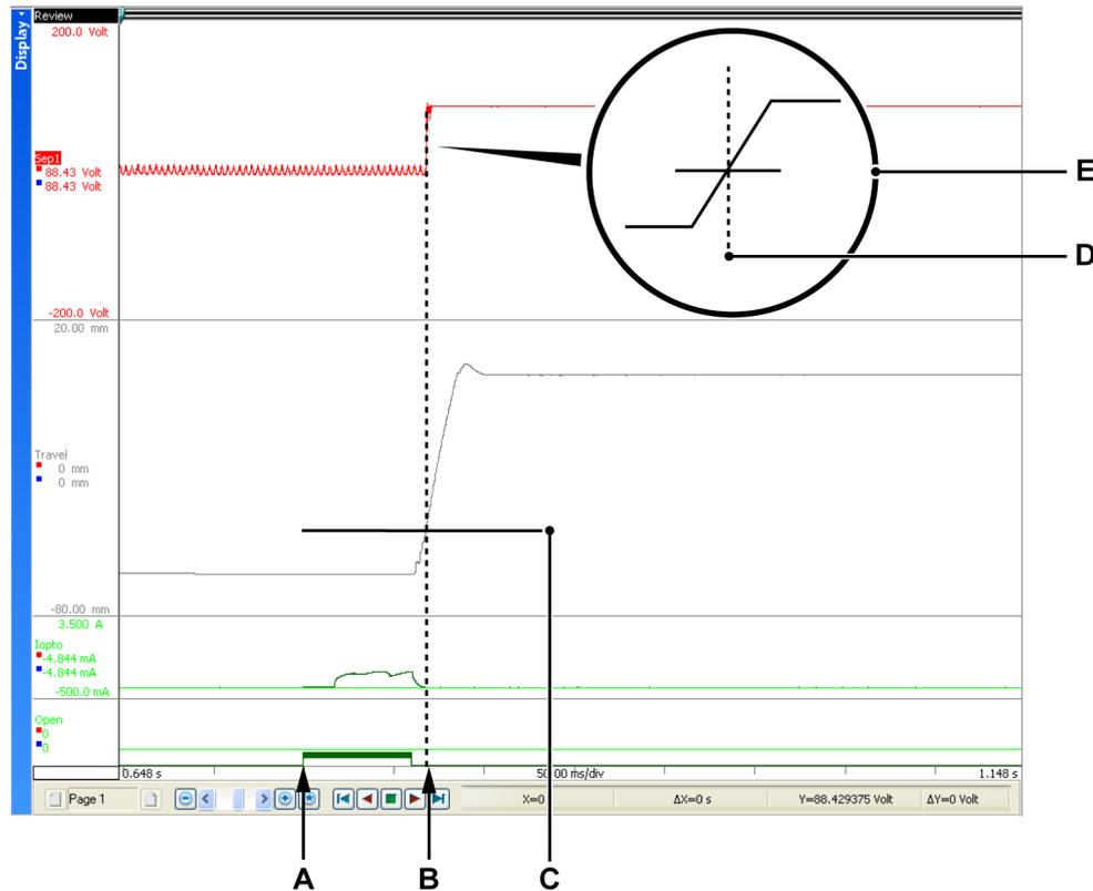
**Figure 4.7:** Display - Close event - Calculations on No-Load
